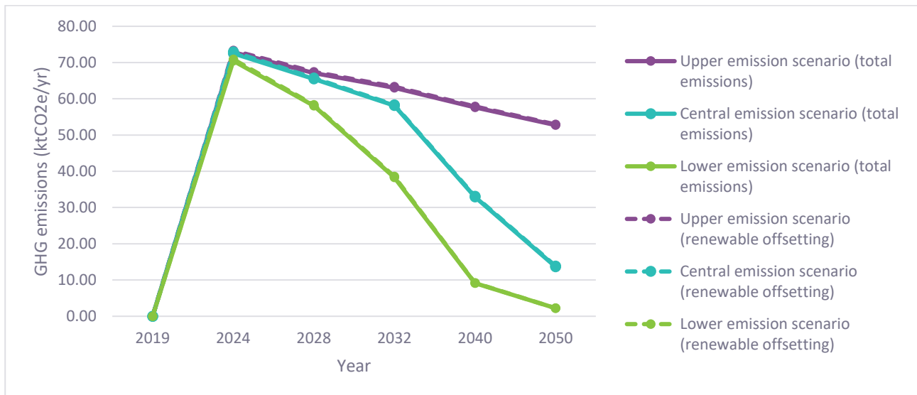
Figure 7A.4 Total GHG emissions (solid line) and residual GHG emissions once offsetting commitments are considered (dashed line) which are assumed to be indicative of the scope of the Luton Borough Council Climate Change Action Plan aim from the Proposed Scheme only.
